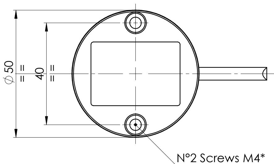
\* MAX tightening torque 2.5Nm
